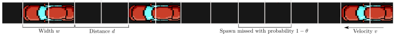
Figure 3.2.: Structure of a street lane in terms of object width w , object distance d , lane velocity v and spawn probability \theta . The distance between two objects is always equivalent to d + i \cdot (w + d) fields where i denotes the number of non-spawned objects between the current and the previous object. This also applies to river lanes in the same manner.
